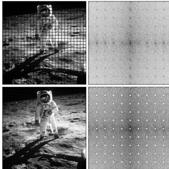
Figure 2: An example of periodic noise removal. The noisy image (upper left) is denoised by taking its 2DFT (upper right), removing local peaks that correspond to the repeating pattern (lower right) and inverting the 2DFT to obtain the denoised image (lower left).
