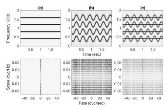
Fig. 4. The top row shows the two sources and their mixture in the time-frequency domain. The bottom row shows the 2D Fourier transform magnitude of the *complex* STFT of the signal. Compare this to Figure 2, which shows the 2D Fourier transform of the *magnitude* STFT of the same signal.
