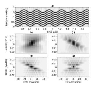
Fig. 5. The effect of 2D-window size on resolution of the scale-rate-domain representation of the magnitude STFT. Panel (a) shows the magnitude STFT of a harmonic, frequency-modulated signal with a fundamental frequency of 200 Hz. Panels (b-e) show the 2D Fourier transform magnitude of the signal over window sizes of  $16 \times 16$ ,  $16 \times 32$ ,  $32 \times 32$ , and  $32 \times 64$  respectively.
