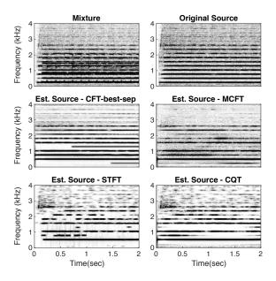
Fig. 8. An example of separation via ideal binary masking with a threshold of  $\gamma=25$  dB for a mixture of C4-clarinet-major trill and C4-flute-vibrato. (a,b) Magnitude spectrograms of the mixture and C4-flute-vibrato. (c-f) Magnitude spectrograms of the estimated source by applying the mask respectively in the CFT-best-sep, MCFT, STFT, and CQT domains.
