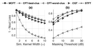
Fig. 11. Mean clusterability for 2D and 4D representations versus similarity kernel width,  $\alpha$  (a) and masking threshold,  $\gamma$  (b). Higher values are better. The results for 2 out of 30 2D window sizes tried in CFT computation are presented: CFT-best-clus (2 × 90) and CFT-worst-clus (32 × 8).
