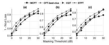
Fig. 12. Mean clusterability versus masking threshold for 2D and 4D representations over (a) three-, (b) four-, and (c) five-source mixture datasets. Higher values are better. Only the results for the best 2D window sizes used in CFT computation  $(2\times 90)$  are presented.
