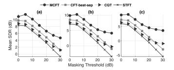
Fig. 10. Mean SDR versus masking threshold for 2D and 4D representations over (a) three-, (c) four-, and (d) five-source mixture datasets. Higher values are better. Only the results for the best two-dimensional window size used in CFT computation  $(4\times64)$  are presented.
