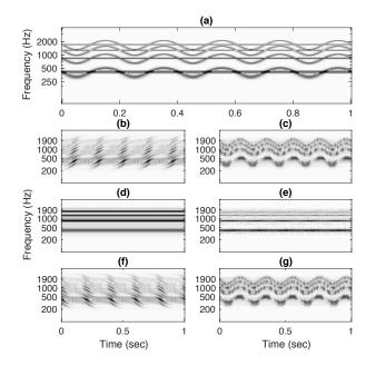
Fig. 7. (a) Magnitude spectrogram of a mixture of two harmonic sources one with and one without frequency modulation. (b,d,f) Magnitude spectrograms of the filtered mixture. Filters are applied to the magnitude spectrogram. (c,e,g) Magnitude spectrogram of the filtered mixture. Filters are first modulated with the mixture phase and then applied to the complex spectrogram.
