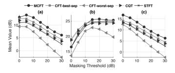
Fig. 9. Measuring Separability for two-source mixtures as a function of masking threshold. Higher values are better. Mean (a) SDR, (b) SIR, and (c) SAR for 2D and 4D representations versus masking threshold,  $\gamma$ . The results for 2 out of 30 2D window sizes tried in CFT computation are presented: CFT-best-sep (4 × 64) and CFT-worst-sep (32 × 4).
