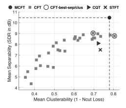
Fig. 13. Mean SDR versus mean clusterability over all samples and masking thresholds for two-source mixtures. The results for all 30 2D window sizes used in CFT computation are presented, along with the results for the MCFT, CQT and STFT. Higher values are better in both dimensions.
