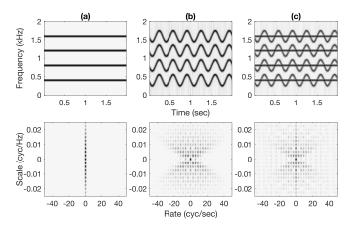
Fig. 2. Two harmonic signals, with and without frequency modulation and their mixture. The two signals have the same fundamental frequency (400 Hz). Columns (a) and (b) show the two separate signals and column (c) shows their mixture. Signals are represented in the time-frequency domain (top row) and in the scale-rate domain (bottom row).
