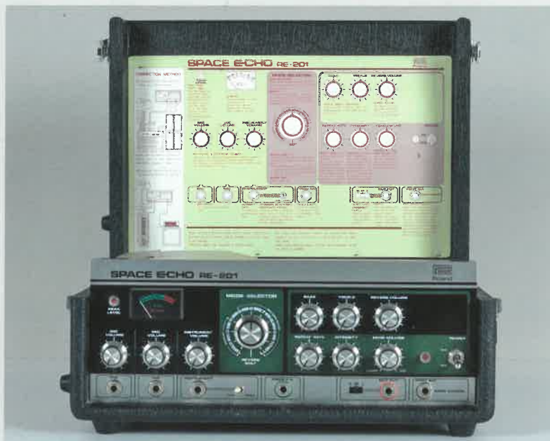
The Roland Space Echo effect had the manual printed inside the lid for easy access during operation. The interface is rather self-explanatory, though.
